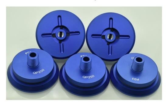
A machined & hard anodized aluminum quarter turn probe with threaded 2.5" OD base plate, a hand knurl and silicone gasket. The QP250 is designed to work with our QD0250 Quick Disconnect set and nylon film bagging.
